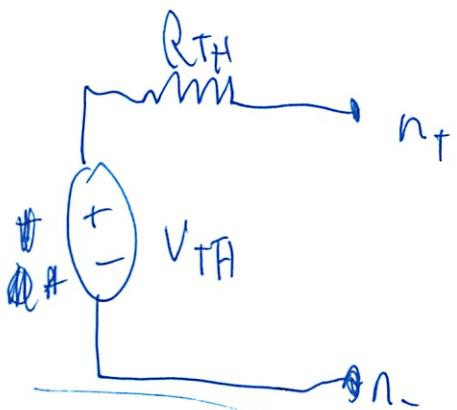
$$i_{SC} = -\frac{V_{TH}}{R_{TH}}$$
