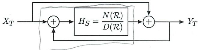
Write a Python function called YinYang that takes a single input parameter HS, which is a SystemFunction that represents  $H_S$ , and returns a SystemFunction that represents  $H_T = Y_T(\mathcal{R})/X_T(\mathcal{R})$ .
