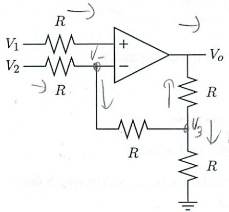
Notice that if we knew the values of  $V_o$  and  $V_2$  then we could calculate the value of  $V_-$ . The resulting value of  $V_-$  will be a linear combination of  $V_2$  and  $V_o$  of the following form:
