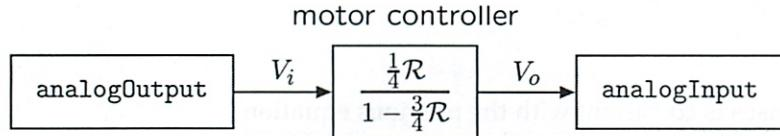
The following code implements a brain that toggles the motor position back and forth by toggling the analogOutput between 0.3 V and 0.7 V.
