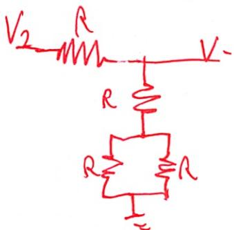
$$V_- = \frac{\frac{3}{2}R}{R+\frac{3}{2}R} V_2 = \frac{3}{5} V_2$$
