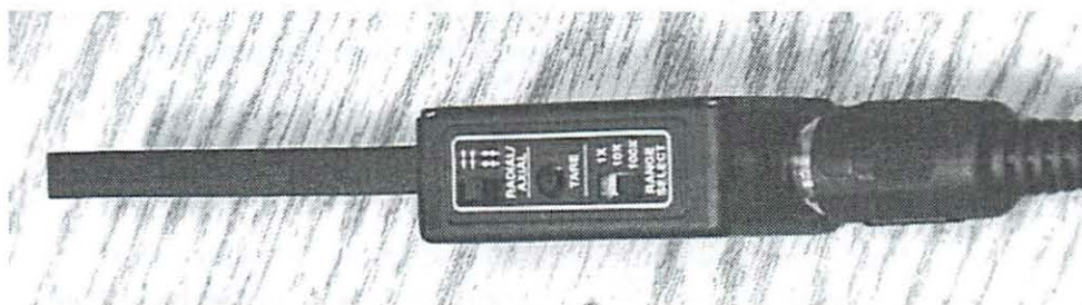
Figure 2 Magnetic field sensor , showing (from right to left) the range select switch, the tare button, and the radial/axial switch, which is set to radial.
