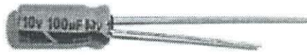
Figure 9 Example of a capacitor. Capacitors on the other hand come in a wide variety of packages and are typically stamped both with their capacitance and with a maximum working voltage.
