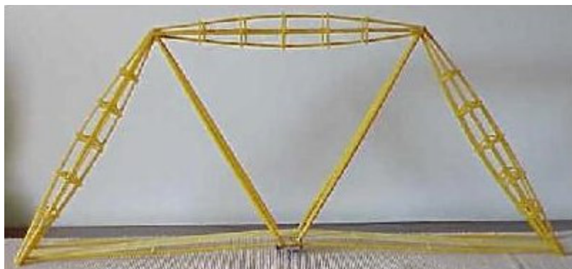
Another use of the Warren truss can be seen here in one of the spaghetti bridges built by students at Johns Hopkins University .
