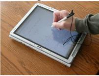
The Fujitsu Tablet PC also has the ability to be written on using a pen. The writing is then converted to electronic ink which appears on the screen. Using the pen to write onto a OneNote notebook is like writing on a big pad of paper.
